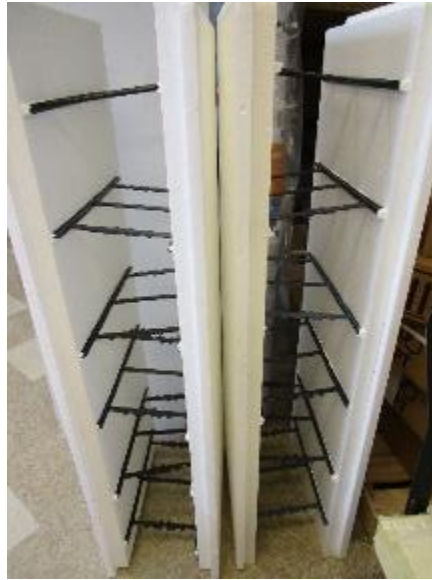
Photo No. 1 ICF Assemblies, As Received
