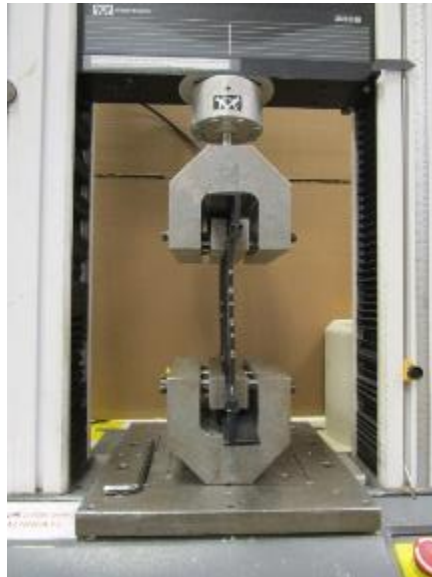
Photo No. 2 Typical Tensile Test Setup Detail
