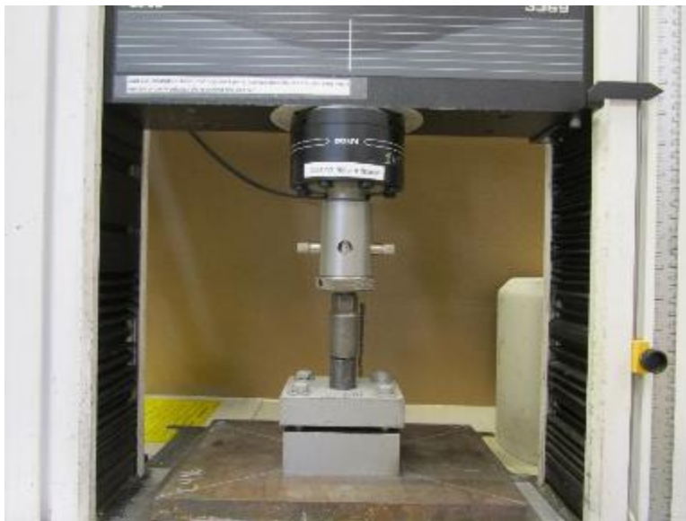
Photo No. 6 Typical Shear Test Setup Detail
