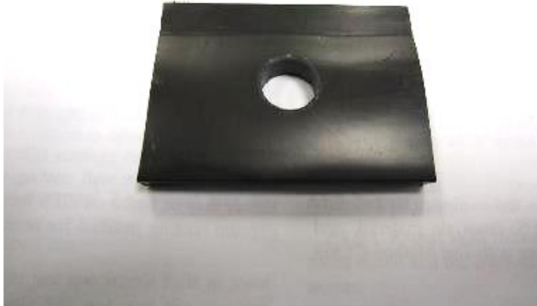
Photo No. 5 Typical Shear Specimen Detail
