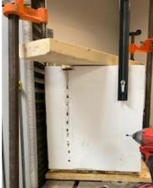
Photo No. 6 Typical Lateral Test Arrangement
