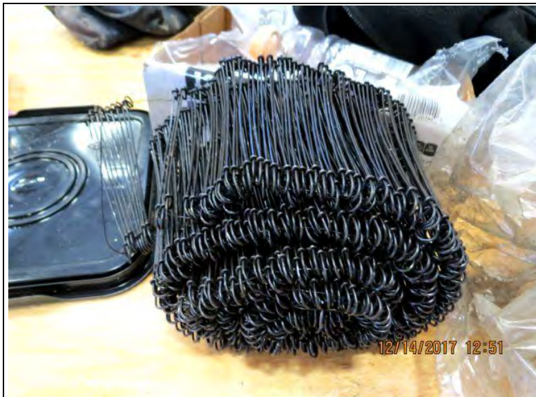
Photo No. 10 Rebar tie-wire
