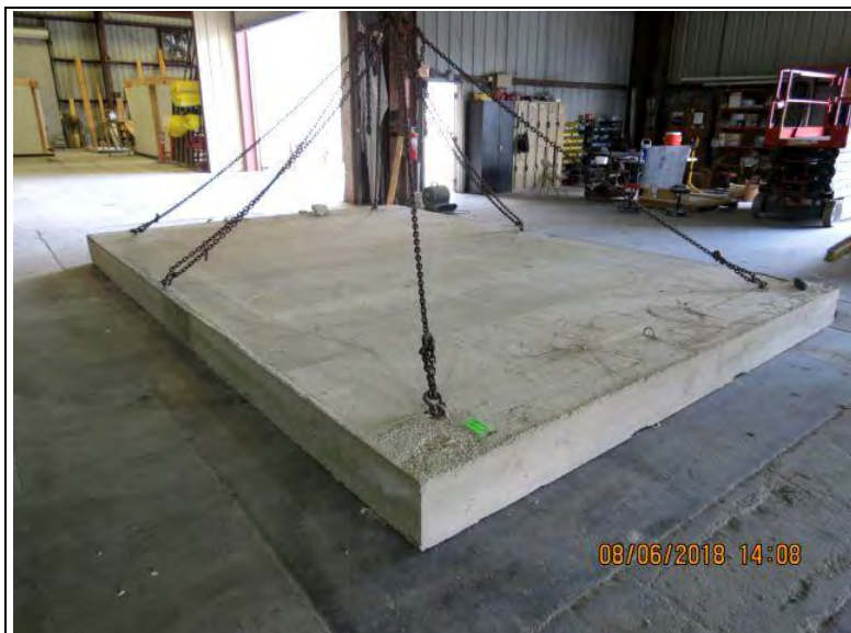
Photo No. 22 Setup into furnace restraining frame
