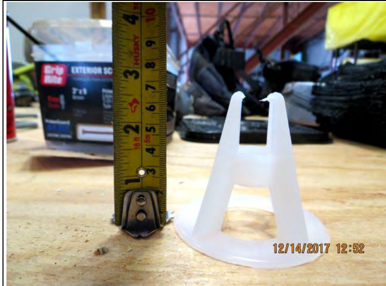
Photo No. 11 Slab reinforcing mesh chair
