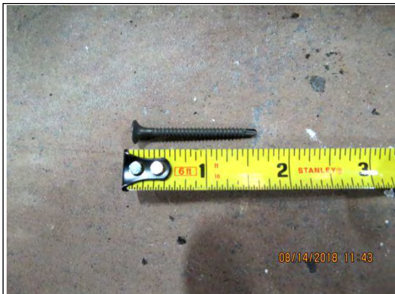
Photo No. 28 Gypsum board fasteners
