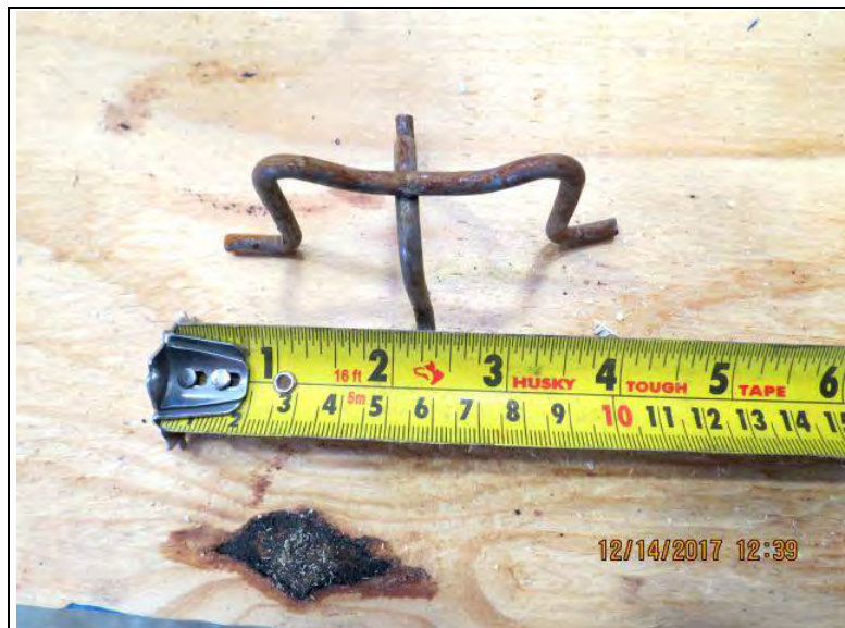
Photo No. 8 Tensioning member rebar chair
