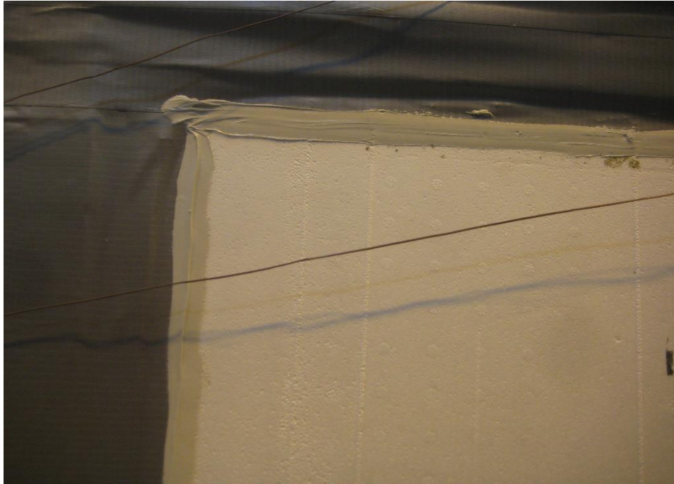
Photo #6, exterior of test unit intalled and sealed with duct tape and caulke
