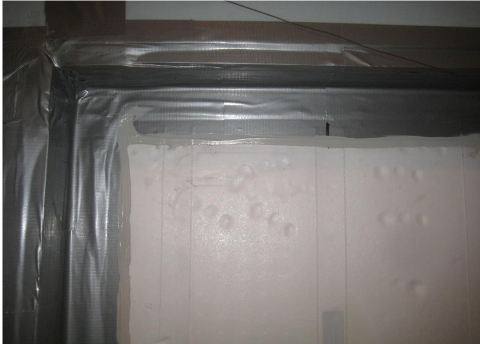
Photo #8, interior of test unit intalled and sealed with duct tape and caulke
